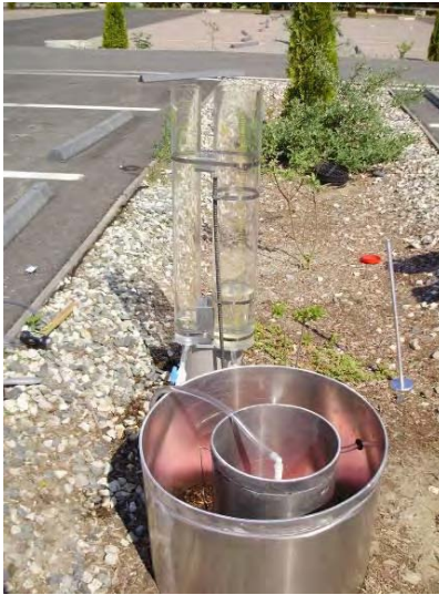
Figure D-2: Double Ring Infiltrometer
