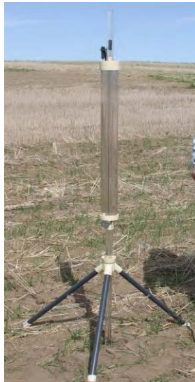
Figure D-3: Guelph Permeameter for Shallow Borehole Permeability
